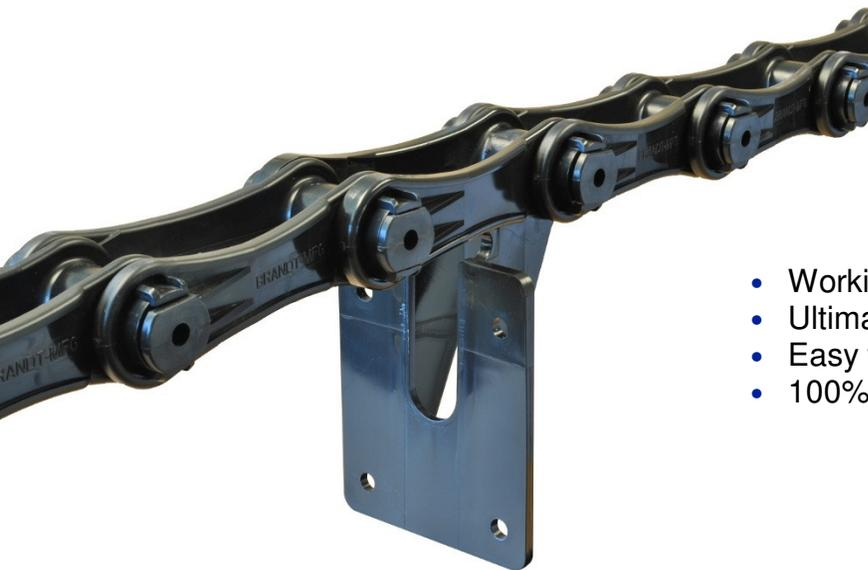
**BRANDT 720 Chain** is a dependable and robust chain designed for use in rectangular sludge collector systems. Made from high modulus engineered resins it does not contain abrasive fiberglass. This results in longer sprocket and system life.
